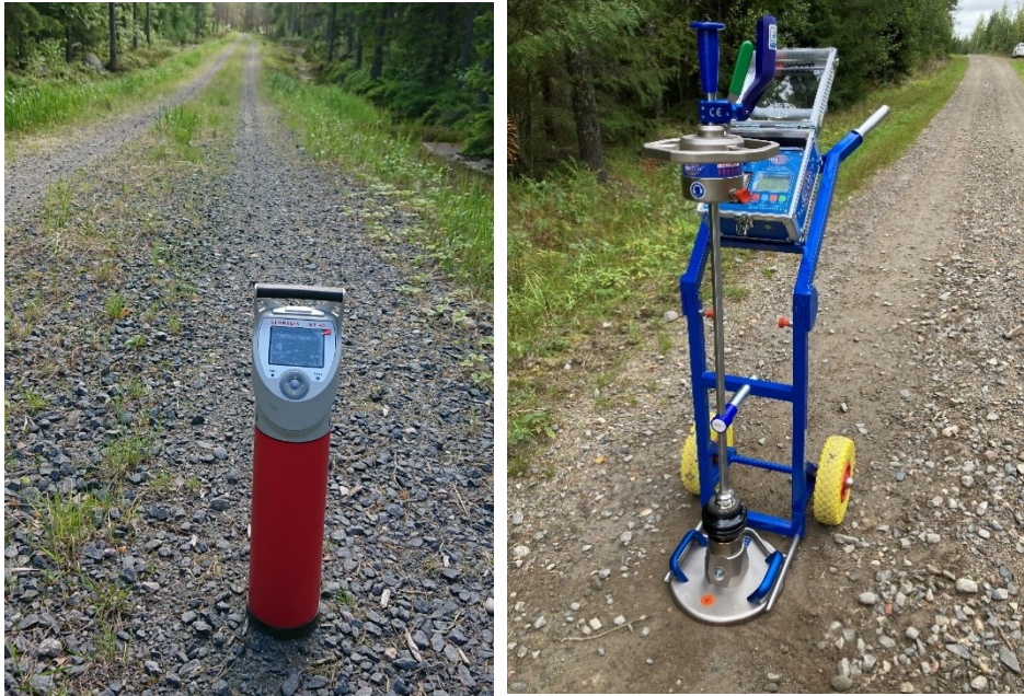
Figure 3. Hand-held gamma-ray spectrometer on the left and Light falling-weight deflectometer (LFW) on the right.
