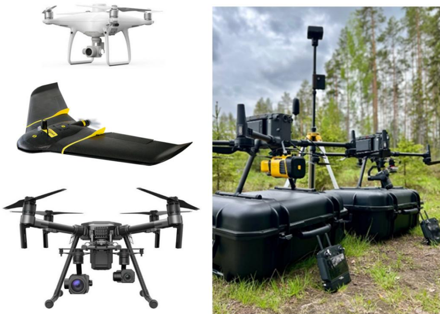
Figure 3. UAV platforms used in this thesis: DJI Phantom 4 RTK, Sensefly eBee plus and DJI Matrice 210 (all left), DJI Matrice 300 RTK (right).
