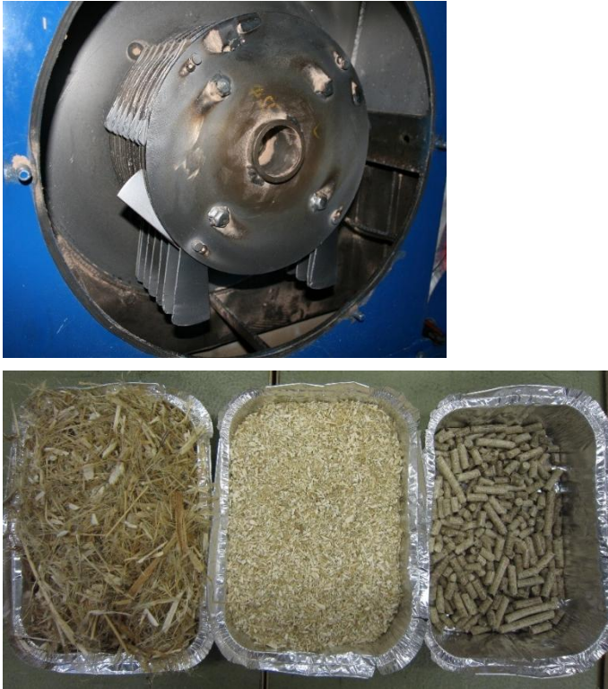
Figure 3. Hammer mill (Miller 20, Miller s.r.l., San Giorgio in Bosco, Italy) used for the hammering process of the giant knotweed and Virginia mallow stalks. Obtained biomass of giant knotweed after pretreatment of stalks (left), hammering process (center), and pellet production (right).
